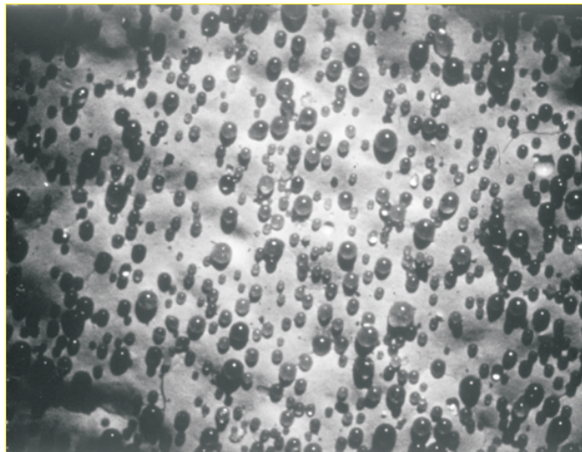
Figure 2.6 Improper bead embedment
