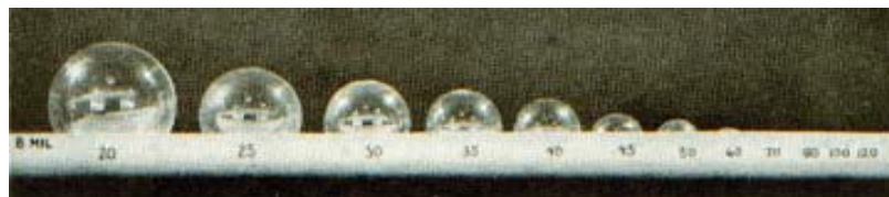
Figure 2.10 Beads in an 8 mil dry line
