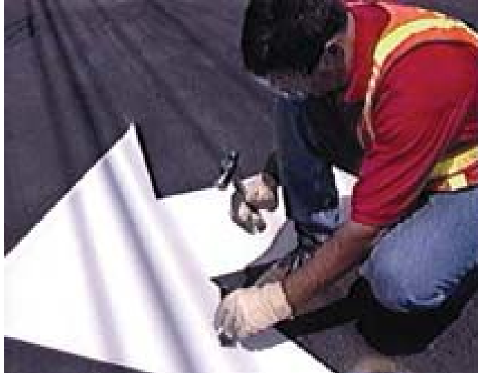
Figure 5.4 Adhesion test being performed
