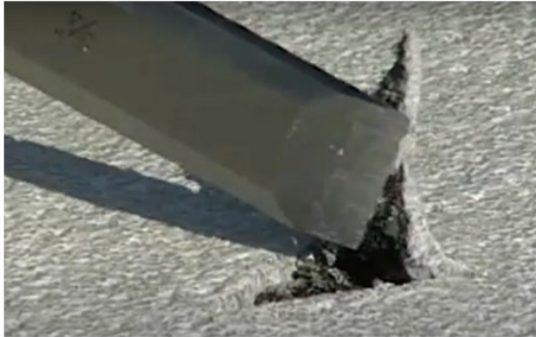
Results of good bonding to the road surface.
