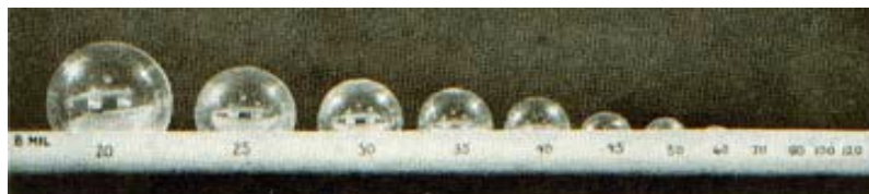
Figure 2.10 Beads in an 8 mil dry line
