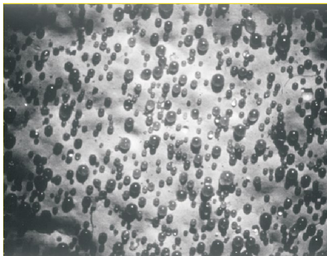
Figure 2.6 Improper bead embedment
